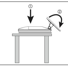
2. Press and hold the monitor with your left hand and at the same time turn the monitor base 90 degrees downwards with your right hand.
