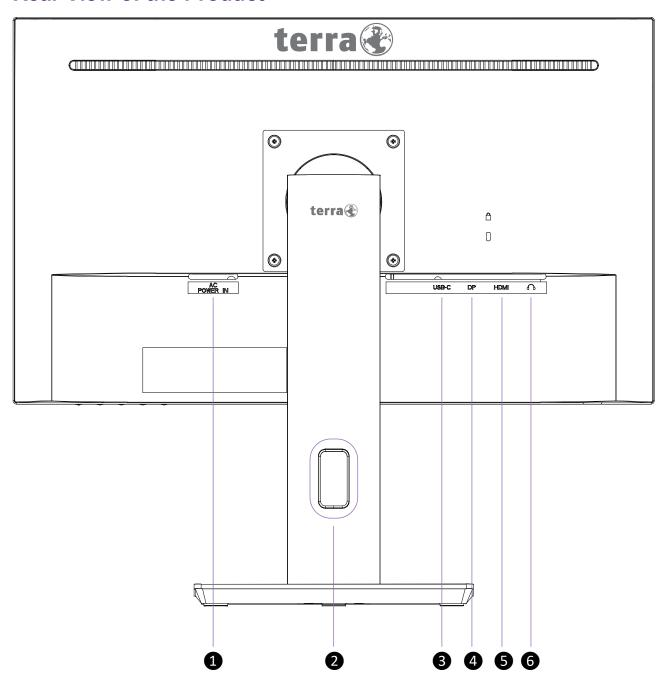
1 Power input 2 Cable Management **USB-C** input 3 Note: USB-C port does not support power charging. DisplayPort input 4 6 **HDMI** input Earphone output Note: Adjustment of the volume control to other settings than the 6 center position may increase the ear-/ headphones output voltage and therefore the sound pressure level.
